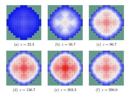
Figure 3: Power distribution maps of the neutron flux at different heights (in cm).
