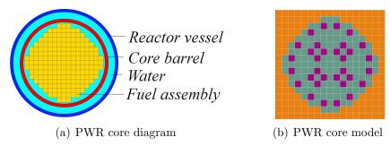
Figure 1: (x, y) core diagram and (x, y) core model of a 3D PWR 900MWe core.
