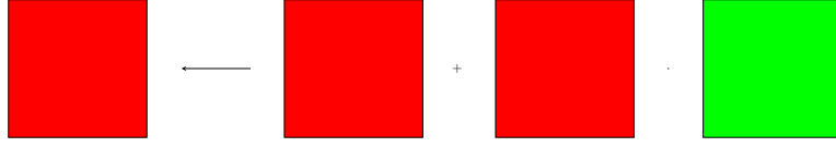
Figure 2.12: A_{\tau,\sigma} is a full matrix, A_{\tau,\zeta} is a full matrix and A_{\zeta,\sigma} is a low-rank matrix.
