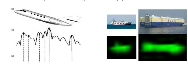
Left: The range profile response (b) of an aircraft (a) and the estimated position of its main scatters (c). Right: Real two dimensional radar video image and its correspondent target.
