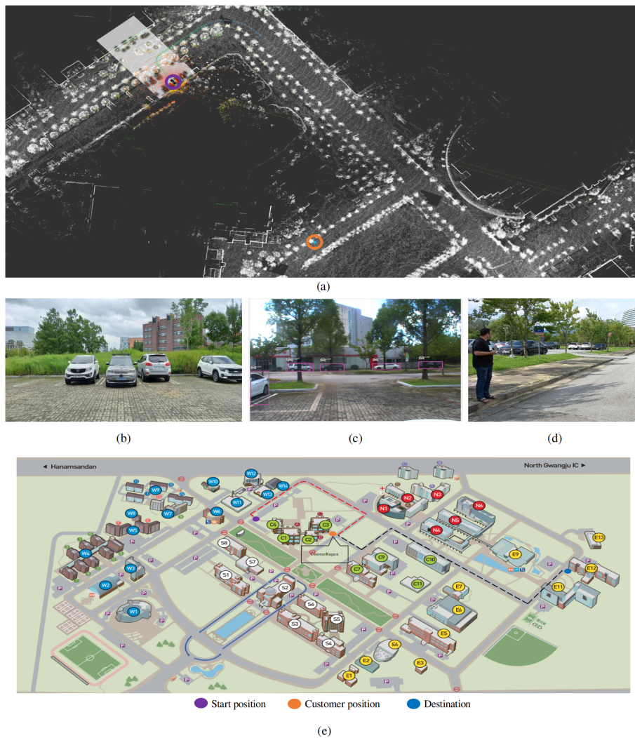
Figure 24. The visualization of autonomous taxi service as an application of our autonomous vehicle. (a) The 3D map shows the start and customer’s pick up position upon receiving the request. (b) Image view of start position. (c) Front-facing camera view from the start position. (d) illustrates that the customer is waiting for the autonomous taxi service. (e) The map of our institute shows the start, customer and destination position (Best viewed in color).
