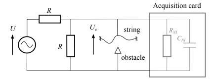
Figure 9: Electric scheme for contact detection.
