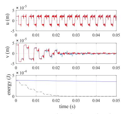
Figure 18: Top and centre: experimental (blue line) and numerical (red line) string displacement along (Oz) (at 1 cm near the edge x=L) and (Oy) (at 2 cm near the edge x=L) with a centered point obstacle and  $B=1.78\times 10^{-5}$ . Bottom: numerical energy of u (blue line) and v (dark dashed line).
