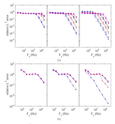
Figure 3: Relative L<sup>2</sup> error versus  $F_s$ , over 3 seconds. Left:  $\alpha=1$ , centre:  $\alpha=1.5$ , right:  $\alpha=2$ .  $K=10^7$  (blue),  $K=10^9$  (red),  $K=10^{11}$  (black) and  $K=10^{13}$  (magenta). (a) N=2, lossless (solid lines) and lossy (dashed lines) stiff string,  $B=1.78\times 10^{-5}$  (b) N=1002, centered point obstacle, lossy stiff string,  $B=1.78\times 10^{-5}$ .
