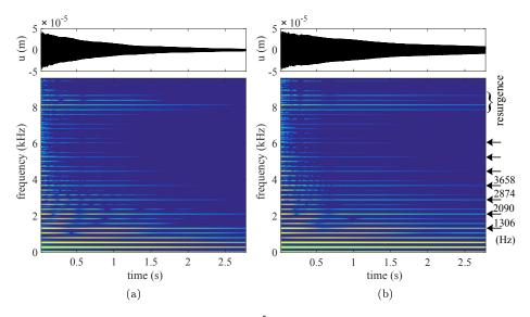
Figure 16: Centered obstacle,  $B=1.78\times 10^{-5}.$  Spectrograms: (a) experimental, (b) numerical.
