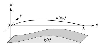
Figure 1: A string of length L vibrating against an obstacle g(x).
