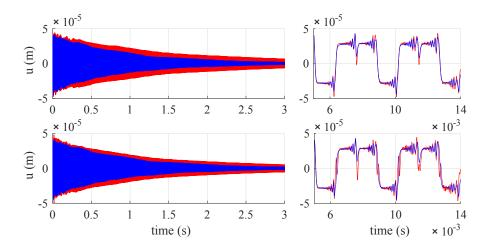
Figure 15: Numerical (red line) and experimental (blue line) displacement signals with a centered point obstacle, with  $B=1.78\times 10^{-5}$ , including contact losses with  $\beta=500$  (top) and  $\beta=1000$  (bottom).
