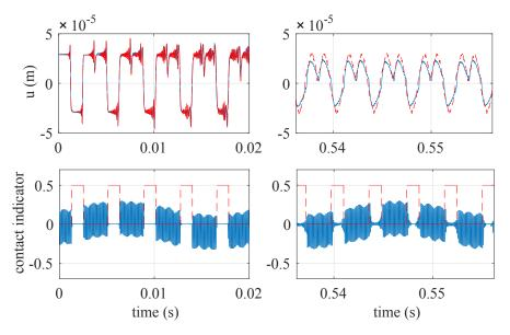
Figure 17: Top: experimental (blue line) and numerical (red dashed line) string displacement with a centered point obstacle,  $B=1.78\times 10^{-5}$ . Bottom: experimental tension between the string and the obstacle (blue line) and numerical contact indicator function (red dashed line).
