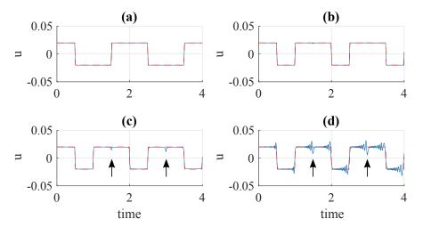
Figure 6: Time signal of the dimensionless string at  $x_m=9L/100$ , comparison of analytical solution for an ideal string (red dashed line), and numerical results (blue line). N=1002,  $F_{s,d}=5000$ . Variables are dimensionless. (a) ideal string without losses or dispersion, and without obstacle. (b) ideal string with obstacle. (c) losses added in the numerical simulation, with obstacle. (d) dispersive lossless numerical string with obstacle,  $B_d=2\times 10^{-5}$ .
