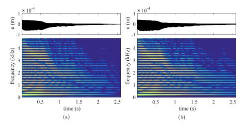
Figure 20: Two point bridge,  $B = 1.78 \times 10^{-5}$ . Spectrograms: (a) experimental, (b) numerical.
