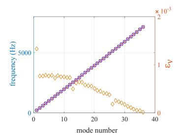
Figure 10: Experimental (red crosses) and theoretical (blue circles) eigenfrequencies,  $\nu_m$  and  $\nu_{th}$  respectively, expanded uncertainty (gray lines) and error indicator (orange diamonds)  $\epsilon_{\nu} = \frac{|\nu_{th} - \nu_m|}{\nu_m}$ , with  $B = 1.78 \times 10^{-5}$ .
