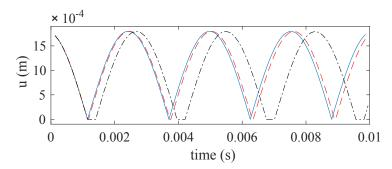
Figure 4: Displacement with  $N-1=1,\,K=10^{13},\,\alpha=1.5.\,F_s\approx 8~\mathrm{kHz}$  (dark dash-dot line), 64 kHz (red dashed line) and 4 MHz (blue line).
