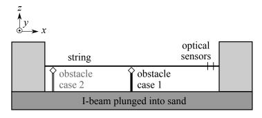
Figure 8: Schematic representation of the measurement frame.
