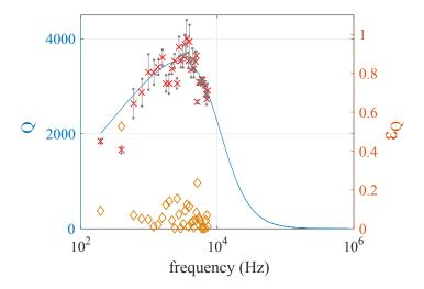
Figure 11: Experimental (red crosses) and theoretical (blue line) quality factors,  $Q_m$  and  $Q_{th}$  respectively, expanded uncertainty at 95 % (gray lines) and error indicator (orange diamonds)  $\epsilon_Q = \frac{|Q_{th} - Q_m|}{Q_m}$ , with  $\delta_{ve} = 4.5 \times 10^{-3}$  and  $Q_{te}^{-1} = 2.03 \times 10^{-4}$ .
