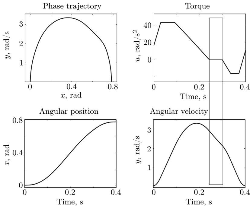
**Fig. 5.** Results for a simulated 1-dof upward movement, with gradient constraints on the torque. The theoretical phase of inactivation of the muscles is shown (rectangular frame). Note that the time to peak velocity (TPV) is 0.47 in this case. It would be equal to 0.53 for the corresponding downward movement, according to experimental findings showing the same directional asymmetries.
