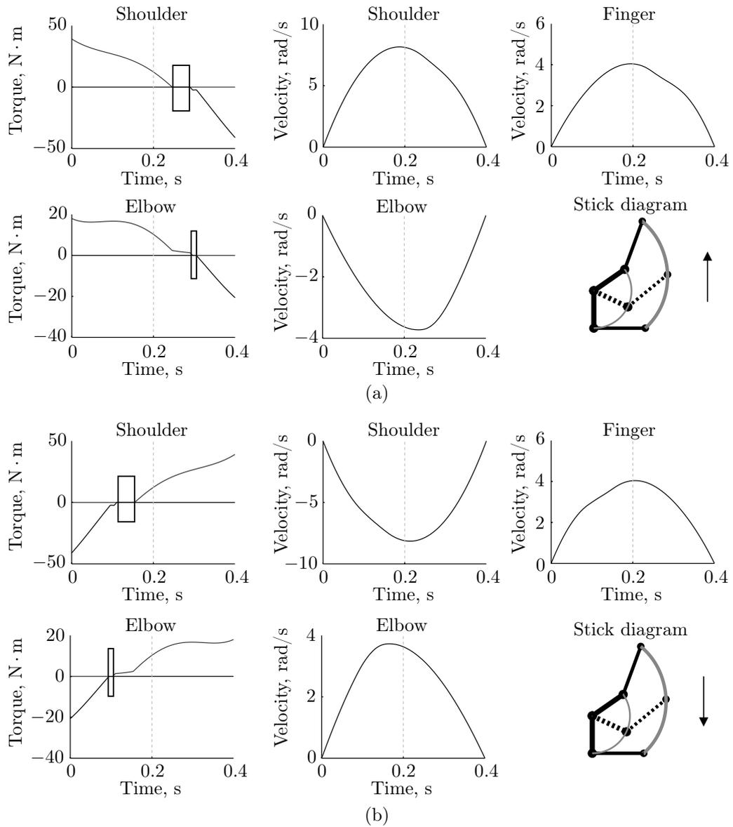
**Fig. 4.** Results for a simulated 2-dof arm movement: (a) upward direction; (b) downward direction. Torques and angular velocities, respectively denoted  $u$  (N·m) and  $y$  (rad/s), are plotted with respect to time (seconds), along with the finger velocity (m/s).
