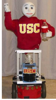
Figure 1: Robot test-bed: Bandit II humanoid torso mounted on the Pioneer mobile base
