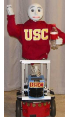
Fig. 1: Robot test-bed: Bandit II humanoid torso mounted on the Pioneer mobile base
