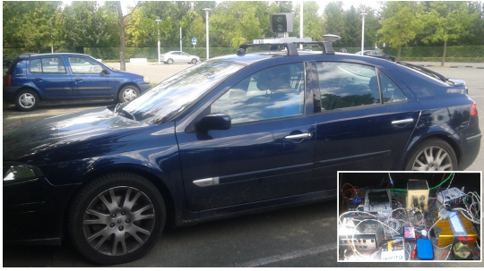
Fig. 2. Test Vehicle used for vehicle tracking experiment. Lidar and GPS are mounted on top of the vehicle and localization system and embedded computers are located in the trunk of the vehicle (see picture inset).
