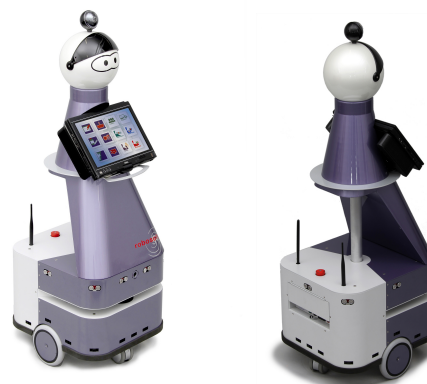
Fig. 1. The mobile robot Kompai (by Robosoft -France) used for interaction.
