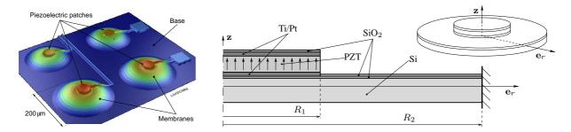
Figure 1. A  $2 \times 2$  resonant membranes matrix biosensor. Cross section of a layered membrane.
